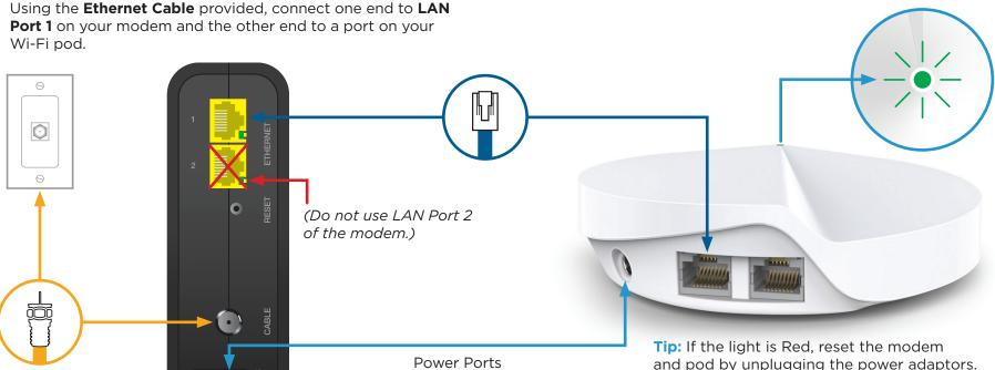
Attach the **Power Cord** to the **Power Port** on your modem, then plug the cord into a nearby power outlet.
